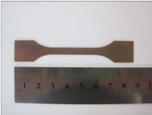
Fig. 9 Tensile specimen of pure copper foil
