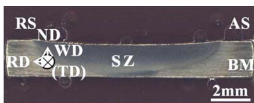
Fig. 1 OM macro image of typical weld cross-section
