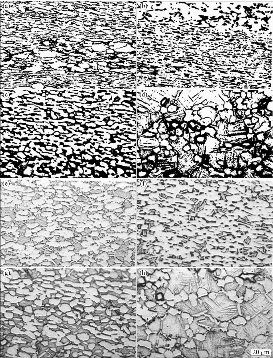
图 1 不同轧制工艺及热处理后 TC4 钛合金板材的显微组织 Fig.1 Microstructures of TC4 alloy sheet after different rolling processes and heat treatments (One-way rolling process (a)–(d), Cross-rolling process (e)–(h)): (a) R; (b) 850 °C, 1 h, WQ+540 °C, 4 h, FC; (c) 900 °C, 1 h, WQ+540 °C, 4 h, FC; (d) 950 °C, 1 h, WQ+540 °C, 4 h, FC; (e) R; (f) 850 °C, 1 h, WQ+540 °C, 4 h, FC; (g) 900 °C, 1 h, WQ+540 °C, 4 h, FC; (h) 950 °C, 1 h, WQ+540 °C, 4 h, FC
