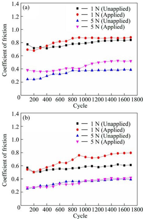
**Fig. 3** Coefficient of friction in terms of travel cycle (aluminum): (a) 0.5 Hz with unapplied or applied magnetic field; (b) 1.0 Hz with unapplied or applied magnetic field
