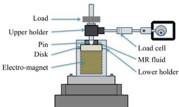
**Fig. 1** Schematic diagram of reciprocating friction wear tester
