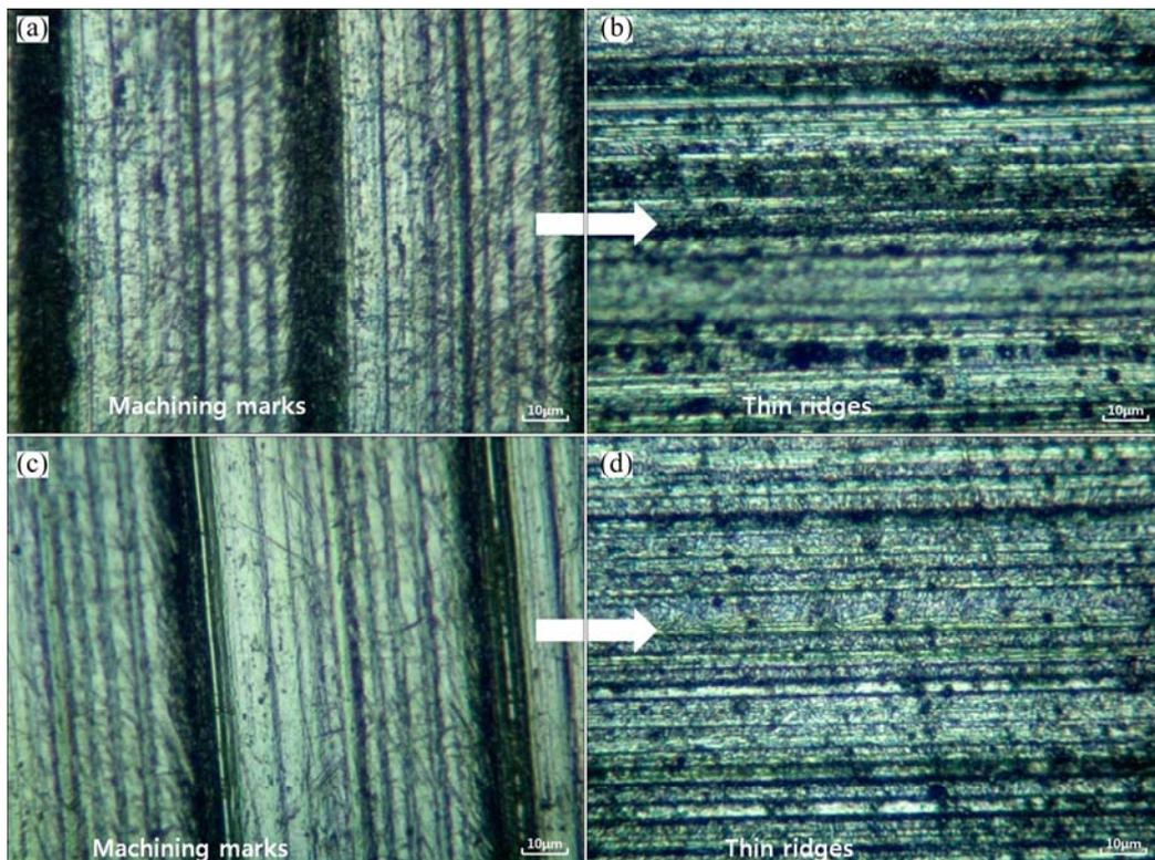
**Fig. 6** Optical images of surface without (a, b) or with (c, d) magnetic field
