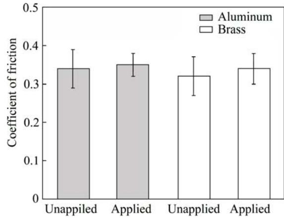
**Fig. 5** Friction coefficient of aluminum and brass in the presence of magnetic field (5 N, 1.0 Hz)
