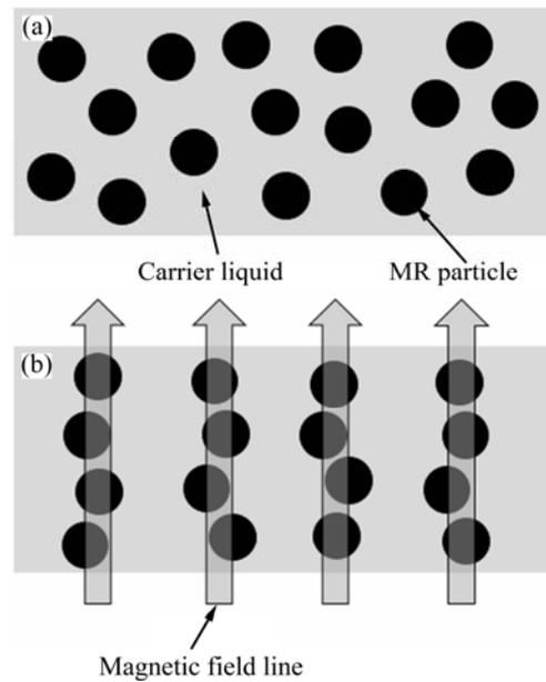
**Fig. 2** Schematic diagram of chain of ferromagnetic particles: (a) Without magnetic field; (b) With magnetic field
