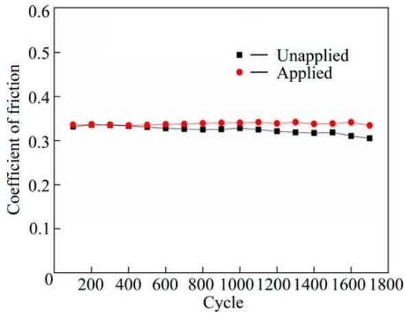
**Fig. 4** Friction coefficient of brass under load of 5 N, oscillating frequency of 1 Hz and magnetic field of 10 mT or no magnetic field
