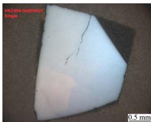
Fig. 6 Oriented \text{Gd}_2\text{PdSi}_3 single crystal
