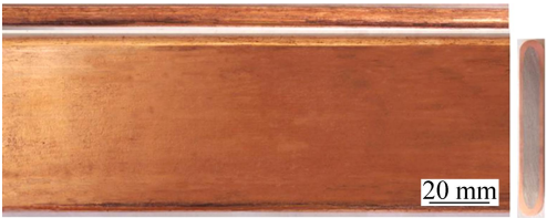
图 1 铜包铝复合扁排宏观形貌 Fig. 1 Macromorphology of copper cladding aluminum flat bar
