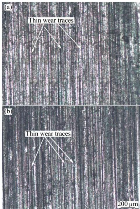
**Fig. 8** Optical photographs of worn surface: (a) Al-Pb alloy; (b) Al-Si alloy
