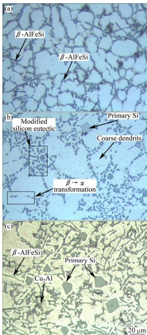
**Fig. 3** Optical microstructural graphs of Al–Si alloy: (a) As-cast; (b) As-cast+T6; (c) 10% forged+T6
