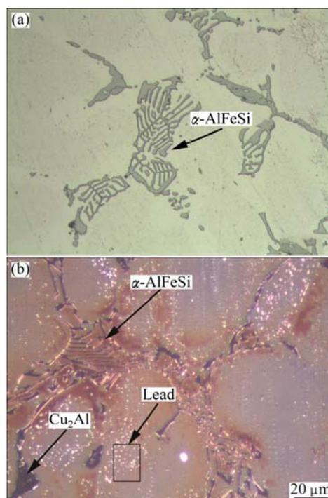
**Fig. 2** Optical microstructural graphs of Al–Pb alloy under day (a) and polarise light (b)
