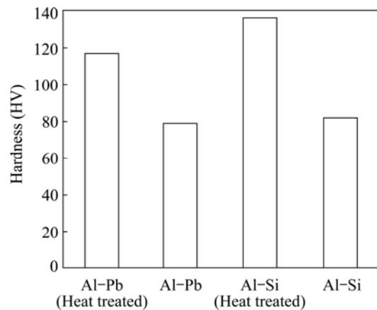
**Fig. 10** Hardness of heat treated (T6) and non-treated Al-Si and Al-Pb alloys
