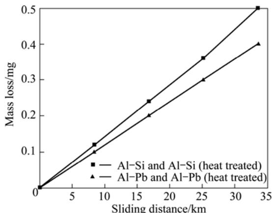
**Fig. 13** Relationship between sliding distance, heat treatment and mass loss for specimens
