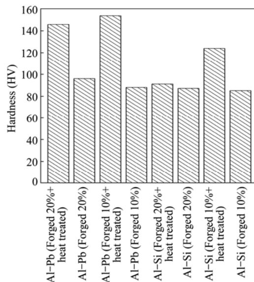
**Fig. 11** Relationship between hardness and forging+heat treatment (T6) for Al-Si and Al-Pb alloys
