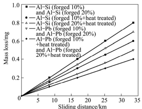
**Fig. 15** Relationship between mass loss, forging, heat treatment and sliding distance for alloys
