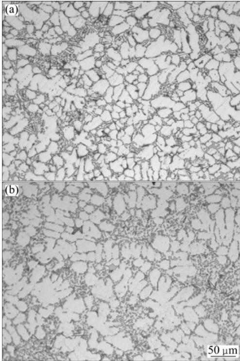
**Fig. 5** Optical microstructural graphs of Al–Si alloy: (a) As-cast; (b) As-cast +T6
