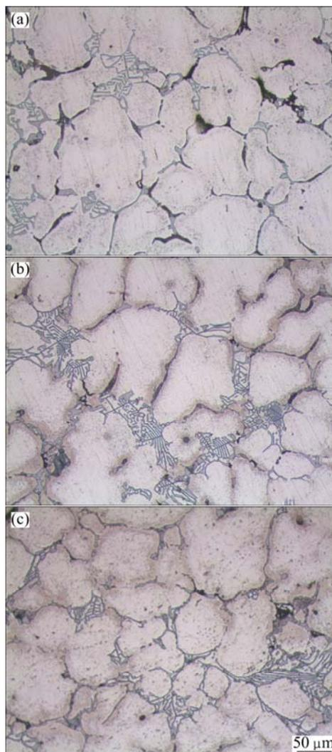
**Fig. 4** Optical microstructural graphs of Al–Pb alloy: (a) As-cast; (b) 10% forged; (c) 20% forged
