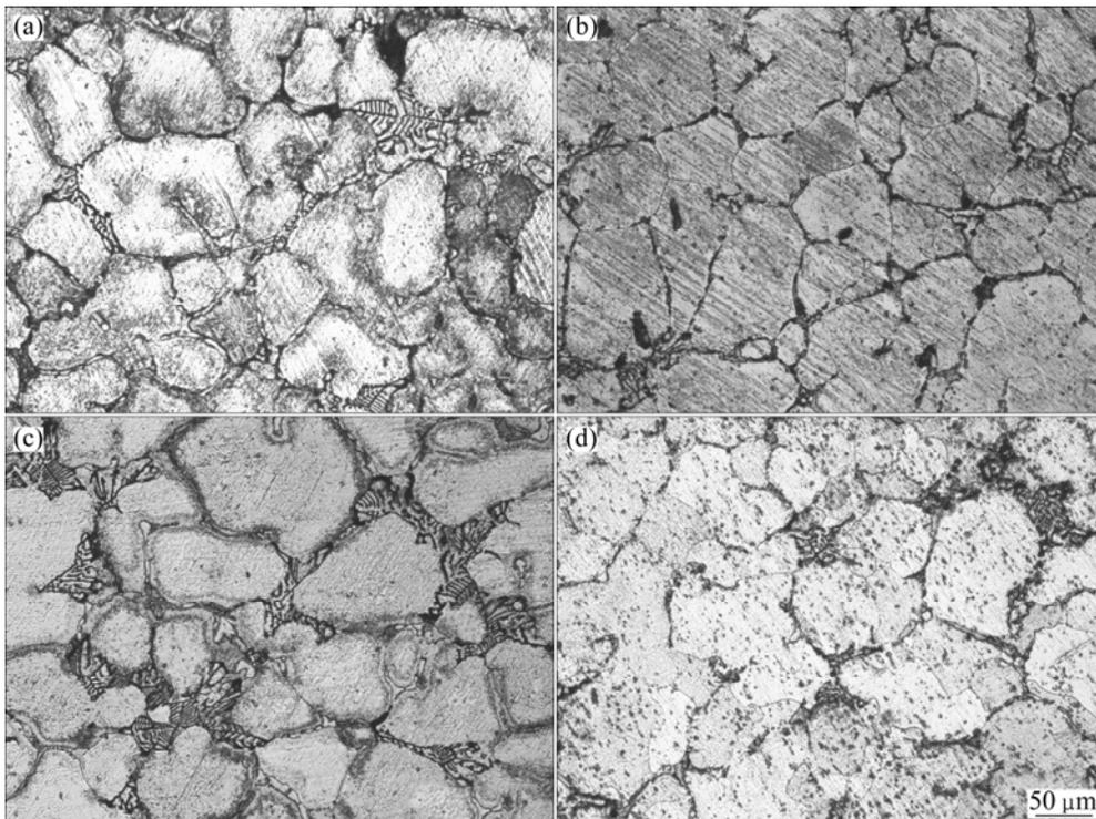
**Fig. 7** Optical microstructural graphs of Al–Pb alloy: (a) As-cast; (b) As-cast+T6; (c) 10% forged; (d) 10% forged +T6
