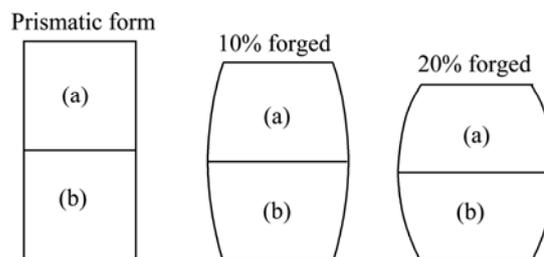
**Fig. 1** Illustration of open-die forging and specimen preparation: (a) Metallography sample; (b) Wear test sample
