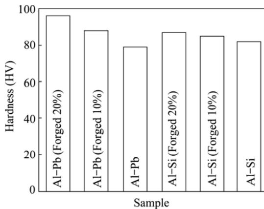
**Fig. 9** Hardness values of unforged and forged materials
