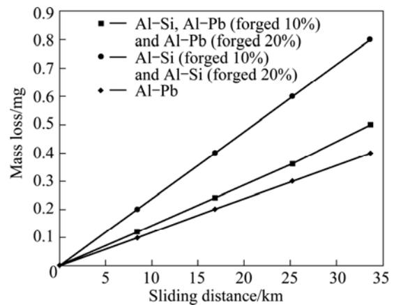
**Fig. 14** Relationship between forging, mass loss and sliding distance for alloys
