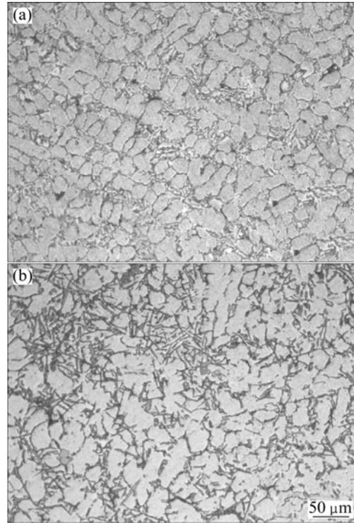
**Fig. 6** Optical microstructural graphs of Al–Si alloy: (a) 10% forged; (b) 10% forged+T6
