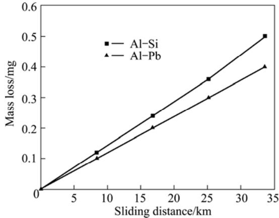
**Fig. 12** Relationship between sliding distance and mass loss of as-cast specimens
