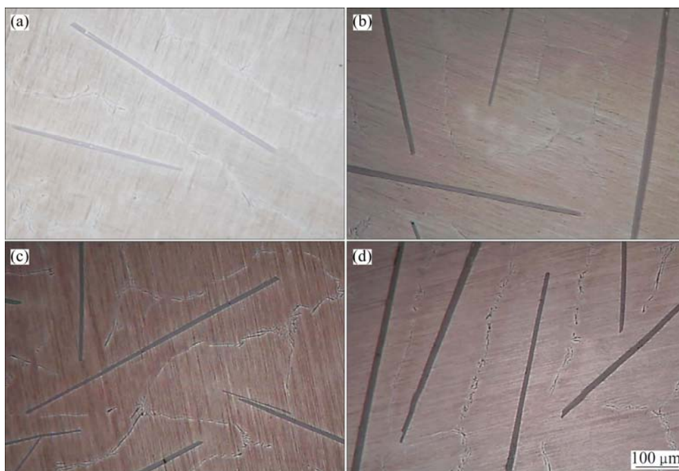
Fig. 6 Metallographic images of Al substrates after being treated at 900 °C for different time: (a) 5 min; (b) 20 min; (c) 30 min; (d) 60 min
