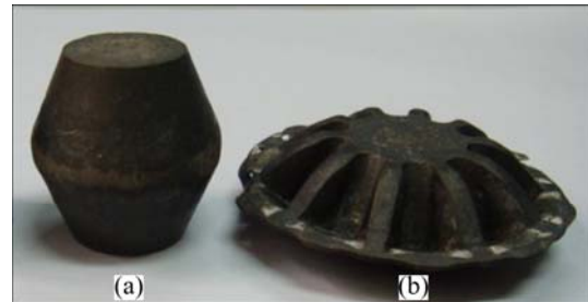
Fig. 8 Photos of preform part (a) and finish forging part (b)
