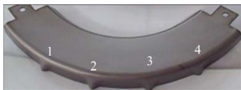
Fig. 10 Rubber forming experimental wrinkles in convex flange with Shore A 90 rubber
