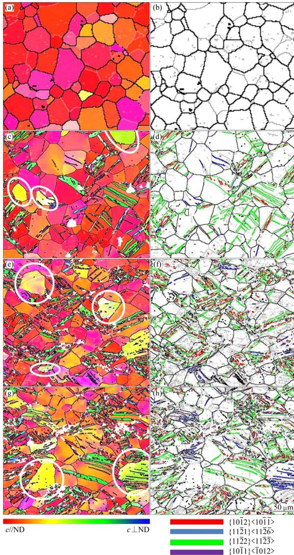
**Fig. 1** Orientation structure and grain boundary maps under different rolling reductions rolled at 77 K: (a), (b) As-received; (c), (d) 5%; (e), (f) 10%; (g), (h) 15%
