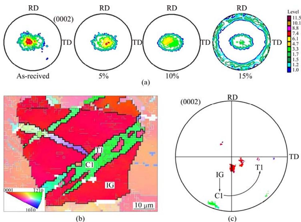
**Fig. 4** Pole figures of as-received, 5%, 10% and 15% samples (a), texture evolution sketch map (b) and (c) (IG, C1, and T1 stand for initial grain, C1 twinning and T1 twinning, respectively)
