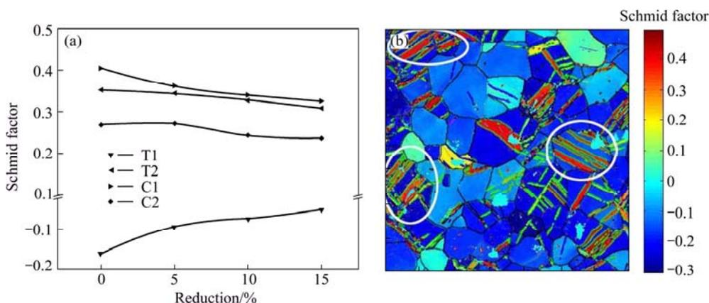
Fig. 3 Schmid factor (a) and SF distribution (b) of T1 at 5% reduction
