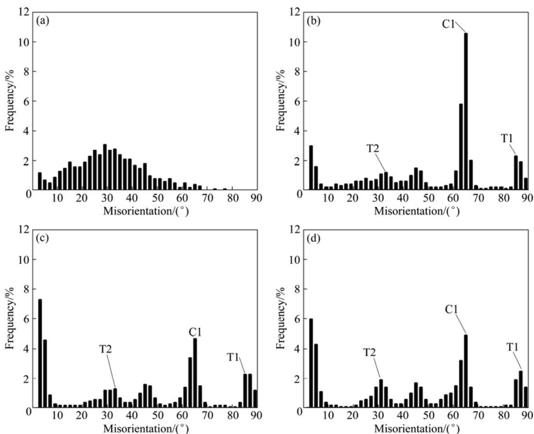
Fig. 2 Misorientation angle distributions of rolled samples under as-received (a), 5% (b), 10% (c) and 15% (d) rolling reduction
