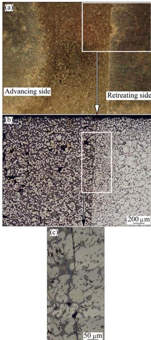
**Fig. 2** Joint microstructure of AZ91 alloy (grooved tool, Mg–25Zn interlayer, 515 °C, 1200 r/min)
