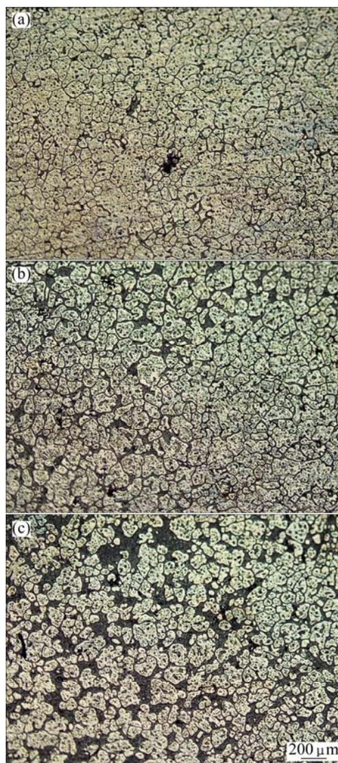
**Fig. 1** Joint microstructures of AZ91 alloy (round tool, without interlayer, 575  $^{\circ}\text{C}$ , 1200 r/min): (a) Base metal; (b) Partially stirred affected zone; (c) Stir zone
