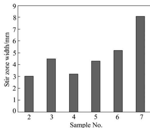
**Fig. 7** Stir zone width of different samples
