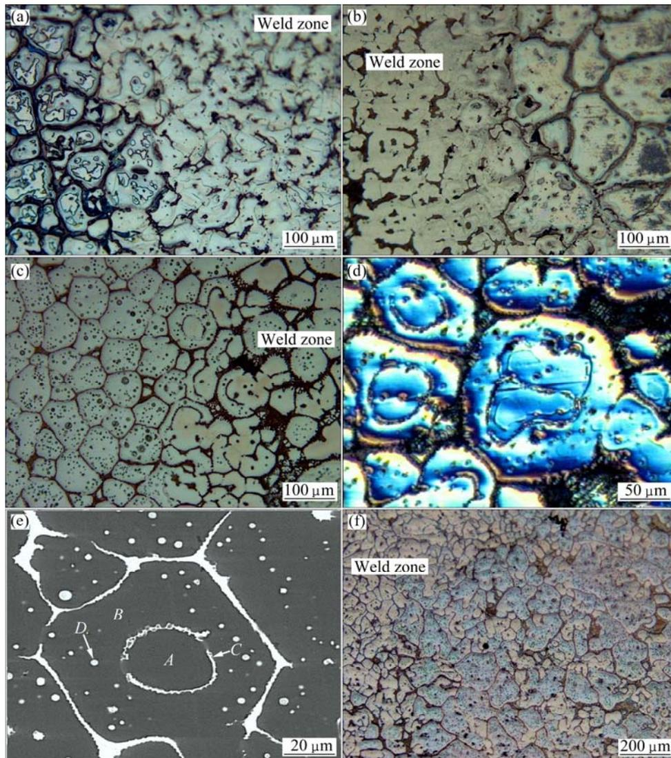
**Fig. 4** Joint microstructure of AZ91 alloy with Mg–25Zn interlayer: (a) Grooved tool, 515 °C, 1600 r/min, interface; (b) Grooved tool, 530 °C, 800 r/min, interface; (c) Round tool, 530 °C, 800 r/min, interface; (d) Round tool, 530 °C, 800 r/min, weld zone; (e) SEM, round tool, 530 °C, 800 r/min, interface; (f) Round tool, 530 °C, 2000 r/min
