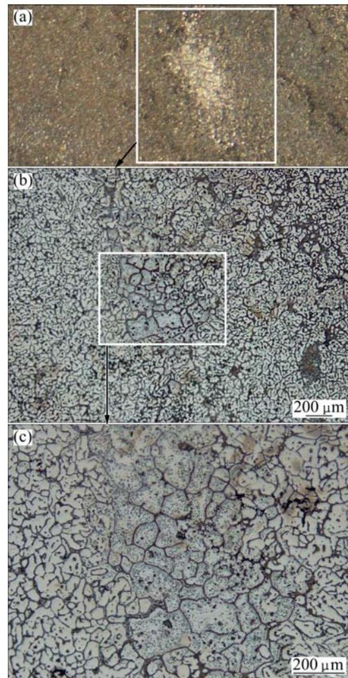
**Fig. 6** Separation of bunched globules from base metal to weld metal (round tool, 530 °C, 1200 r/min)
