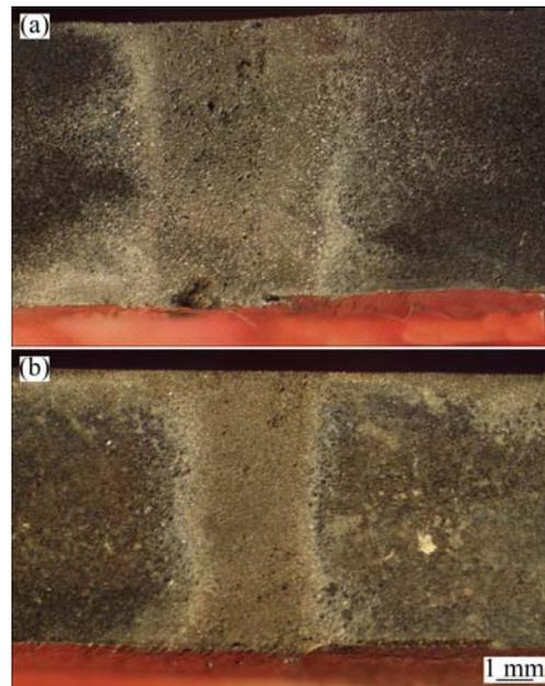
**Fig. 3** Joint macrostructure of AZ91 alloy: (a) Grooved tool, Mg–25Zn interlayer, 515 °C, 1600 r/min; (b) Grooved tool, Mg–25Zn interlayer, 530 °C, 800 r/min
