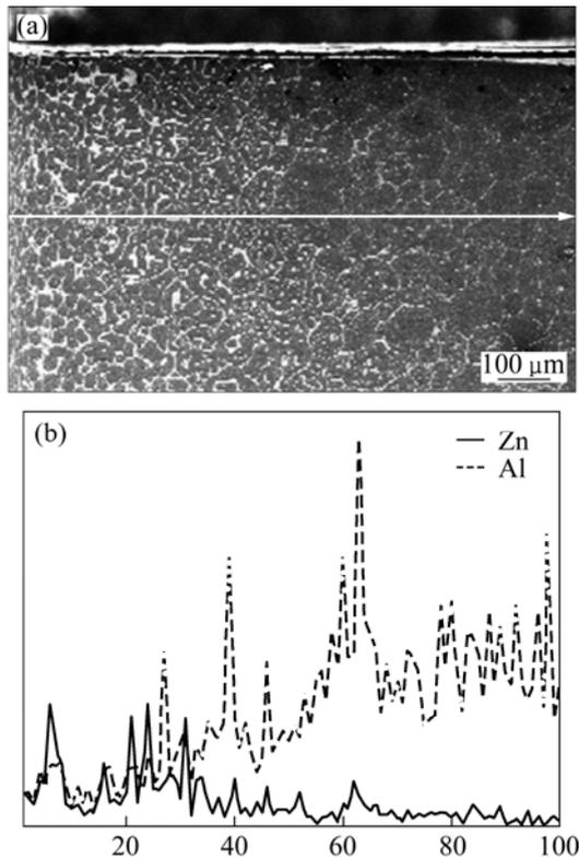
**Fig. 5** SEM image (a) and elemental line scan (b) of weld metal to base metal (round tool, 530 °C, 800 r/min)
