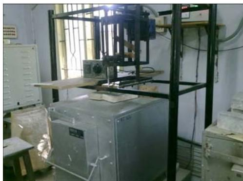
Fig. 1 Experimental setup used for stir casting
