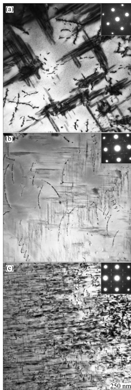
**Fig. 3** TEM images of *S* phases in 2524 alloy aged to peak hardness at 170 °C with various stresses: (a) 0; (b) 173 MPa; (c) 250 MPa
