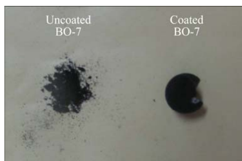
Fig. 7 Macrographs of uncoated and coated BO-7 specimens after oxidation at 873 K in air for 120 min
