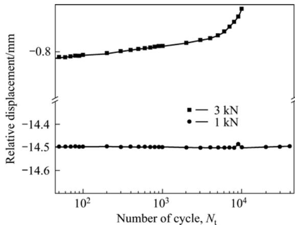
**Fig. 6** Maximum relative displacement of force amplitude with 1 kN and 3 kN
