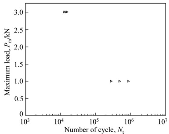
**Fig. 5** Fatigue life of FSSW AZ31 sheet joints
