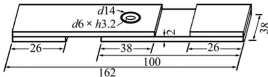
Fig. 2 Test specimen for fatigue test (unit: mm)
