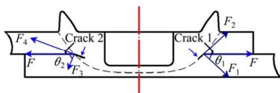
**Fig. 9** Fracture mechanics analysis of FSSW joint under action of cyclic force
