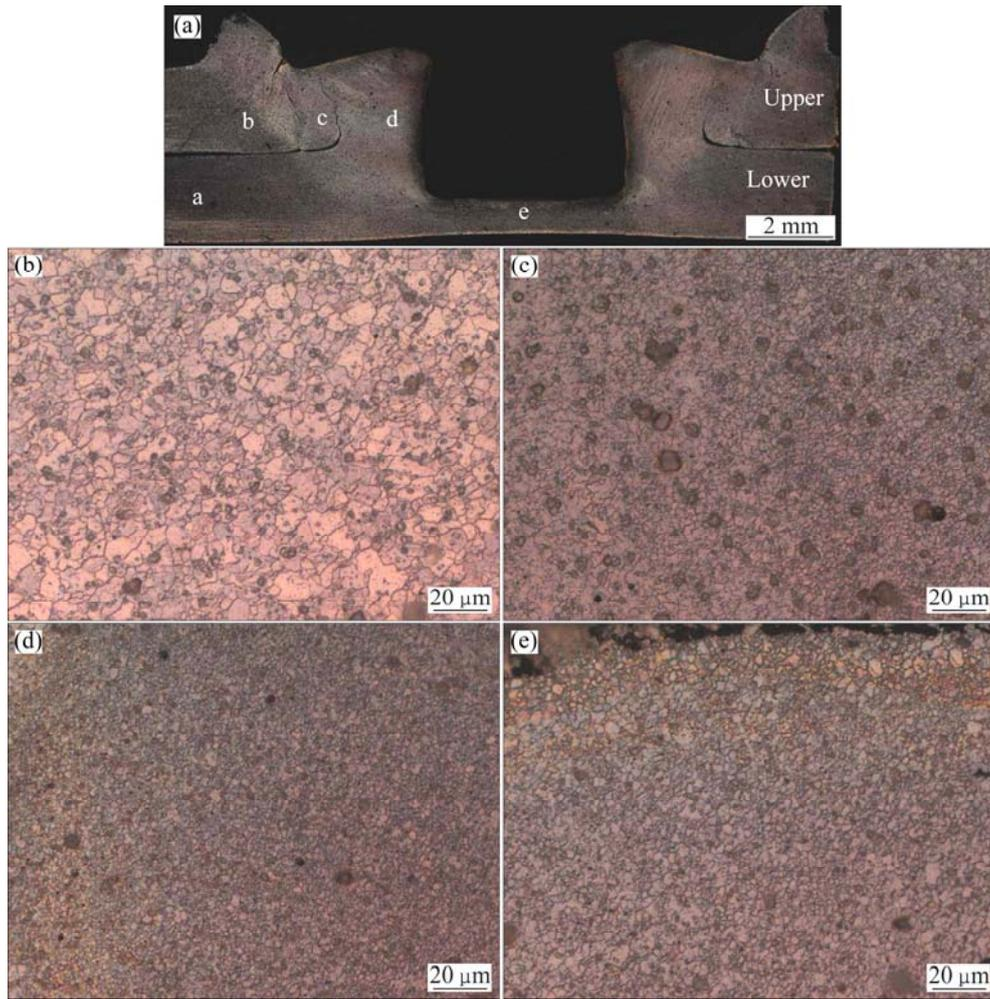
**Fig. 3** Macroscopic structure of transverse section through center of FSSW joint and microstructures of different zone at FSSW joint of AZ31 sheets: (a) Macroscopic structure of transverse section of FSSW joint (a—Base metal; b—Heat-affected zone; c—Thermo-mechanical zone; d—Stirred zone; e—Stirred zone below); (b) Microstructure of heat-affected zone; (c) Microstructure of thermo-mechanical zone; (d) Microstructure of stirred zone; (e) Microstructure of stirred zone below
