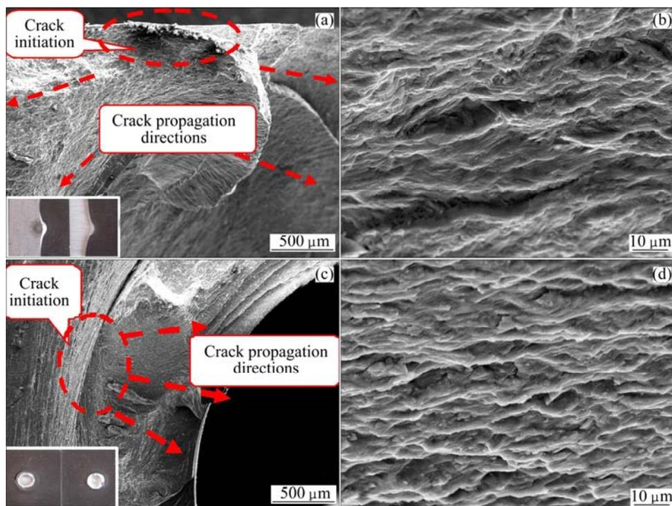
**Fig. 7** Fatigue fractures and crack propagation area characteristics of FSSW AZ31 magnesium alloy sheet joints: (a), (b) 1 kN; (c), (d) 3 kN
