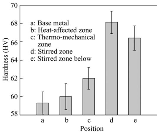
**Fig. 4** Typical hardness of different zones
