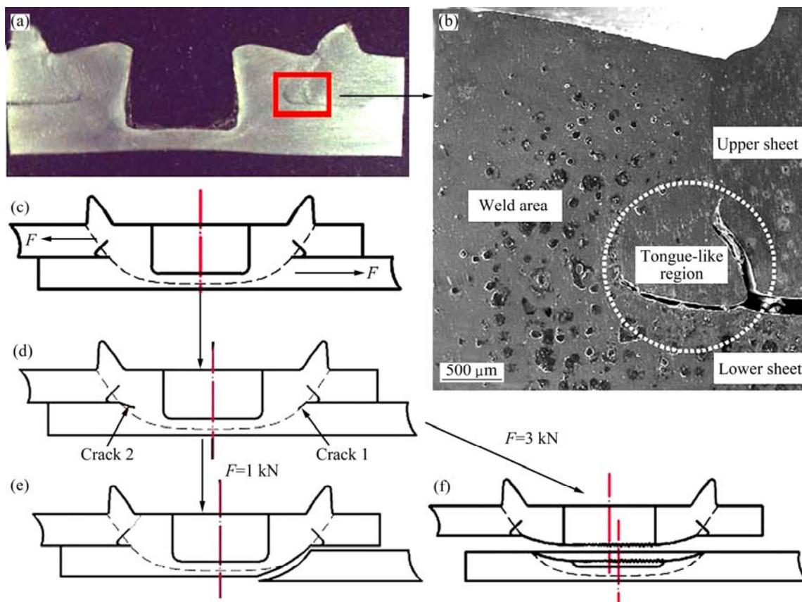
**Fig. 8** Fatigue failure mechanism of FSSW AZ31 alloy sheet joints: (a) Macro-photograph of transverse section through center of FSSW joint; (b) Microstructure of stirred zone; (c) Before fatigue test; (d) Primary stage of crack propagation; (e) failure mode when  $F=1$  kN; (f) Failure mode when  $F=3$  kN
