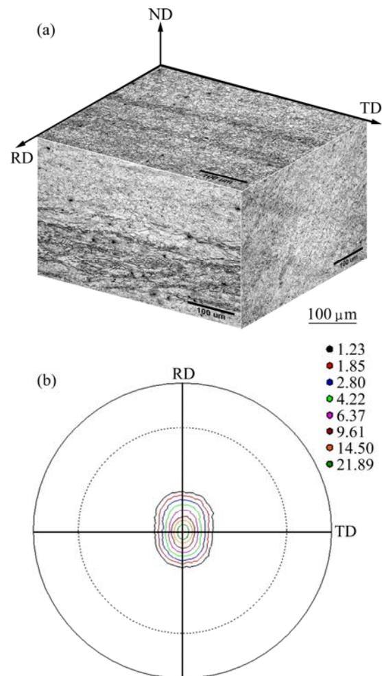
**Fig. 1** Microstructure of rolled AZ31 sheet: (a) Microstructure observed in three planes; (b) {0002} pole figure of rolled sheet
