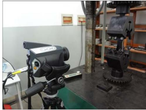
**Fig. 2** Infrared system in fatigue test
