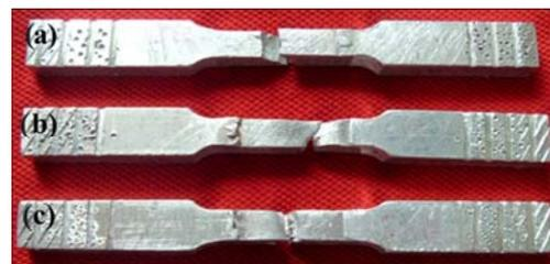
**Fig. 8** Failure regions of dissimilar FS welded aluminum alloy at welding speed of 36 mm/min (a), 90 mm/min (b) and 63 mm/min (c)
